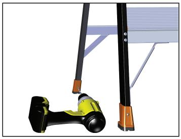
B1. Start by drilling out the clinches of the rivets. Take special care not to damage the fiberglass rails.
